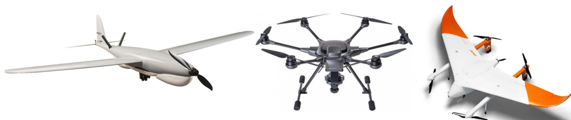
Figure 1. Three categories of drones: with the fixed wing on the left (Sky-watch) [29], multirotor drone in the center (Yuneec) [30], and a VTOL drone on the right (Avy) [31].
