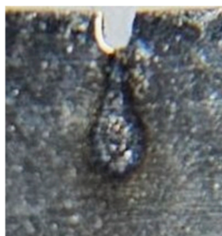
Figure 4. Optical image of the crack healed by six current pulses.
