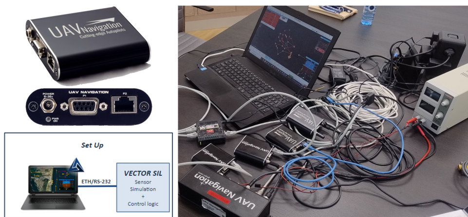
Figure 9. Pictures of the SIL simulation environment provided by UAV Navigation, featuring the VECTOR-SIL and Visionair GCS Software.
