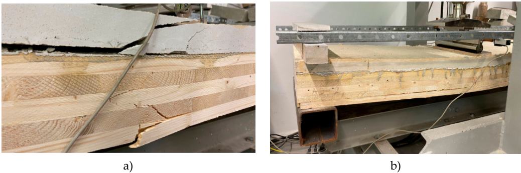
Figure 17. The failure mode of the third group specimens: a) sub-group BS; b) sub-group AS.
