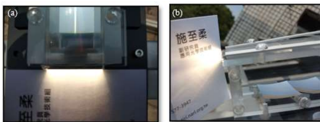
Figure 10. The light emission situation of the light-guide plate of the PT-SACM array. (a) Horizontal light emission, and (b) vertical light emission.
