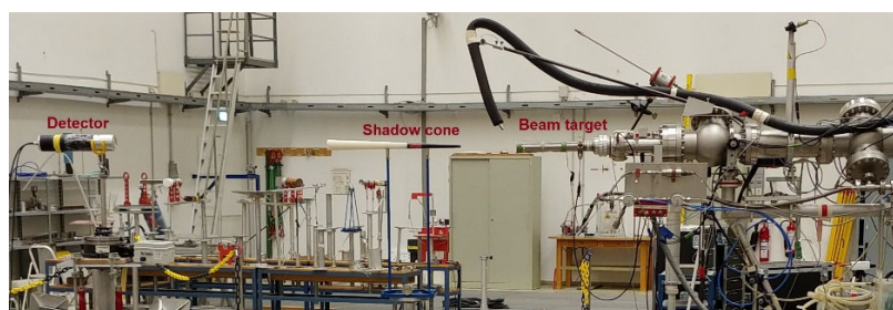
Figure 2. The experimental arrangement in the low-scatter hall. Position of the detector (on the left-side) and the beam target (on the right-side) as used for the measurements. In between there is a shadow cone.
