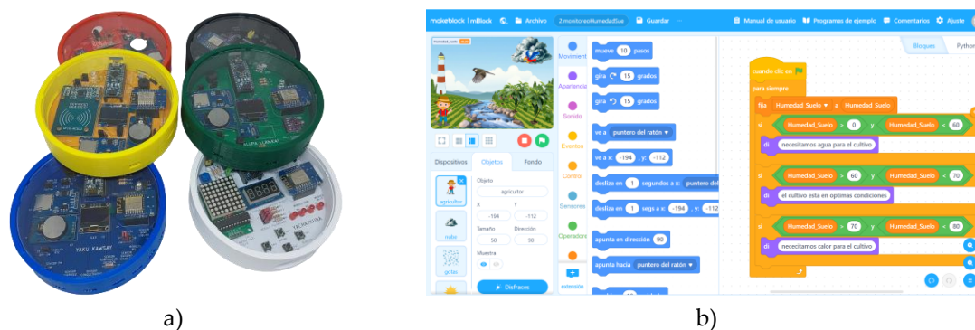
Figure 2. STEM Educational Kit with Visual Programming Environment: a) Six educational electronic boards and b) mBlock visual programming interface.
