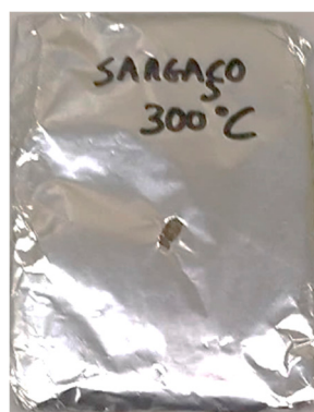
Figure 4. Aluminium foil envelope for biomass carbonization.
