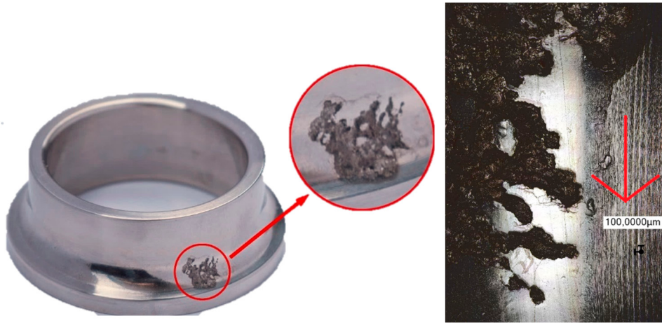
Figure 10. Example for Cold Formed bearing damage.
