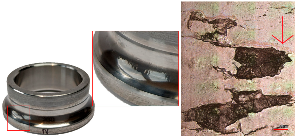
Figure 9. Example for Standard bearing damage.
