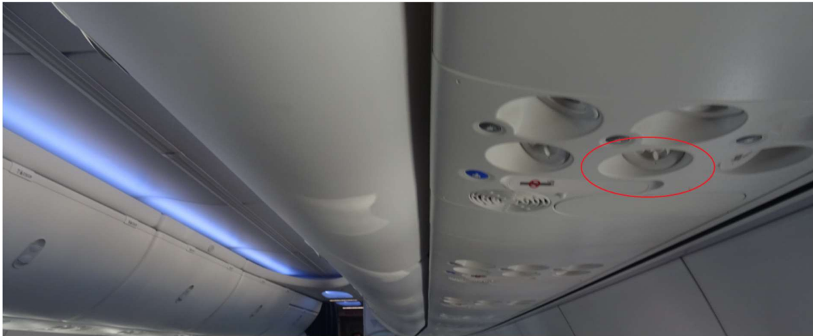
Figure 1. Air vents located in the ceiling of the aircraft cabin. The location of measurement of supply air parameters using the Testo recorder is marked in red.
