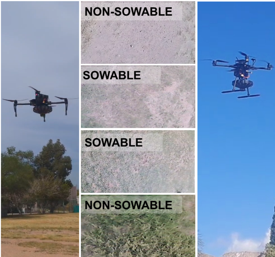
Figure 8. System field evaluation mounted in a DJI Matrice 100 drone (left), and a Holybro x650 drone (right). Four images analyzed by the algorithms classified as sowable and non-sowable.
