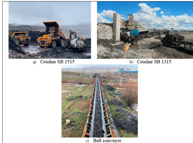
Figure 3. Parts of CCS system at the open pit Gacko (private archive).
