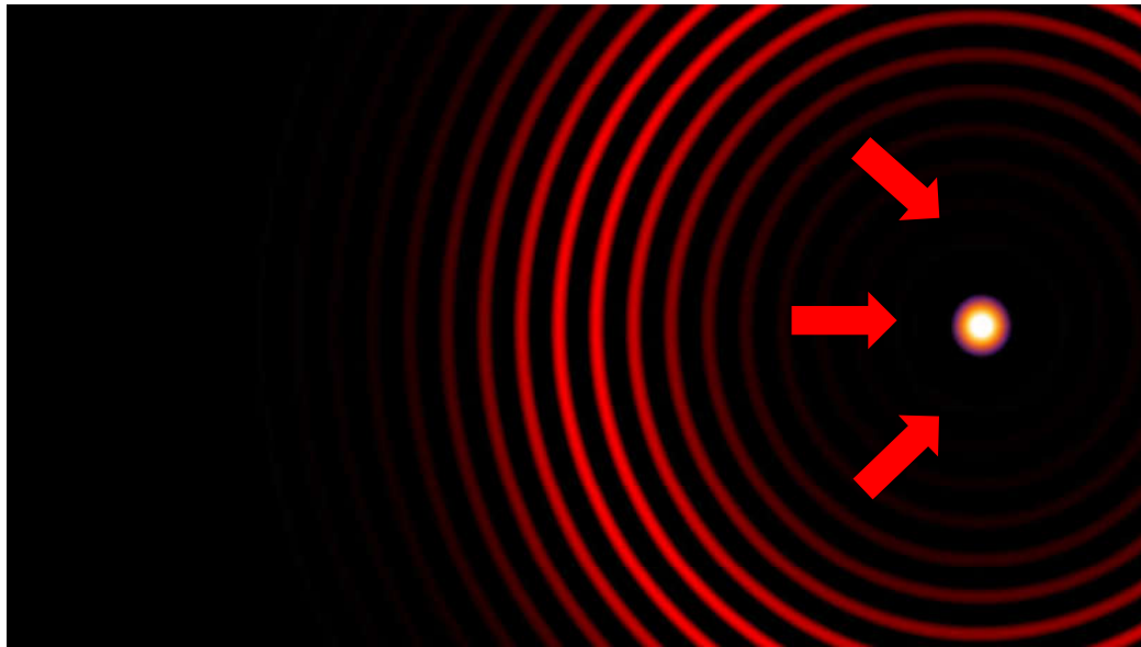
Figure 4. Vector Potential Advanced Wave, generated by the current in the Absorber atom, seen in the x-y plane, looking down the z axis from above. The wave propagates inward toward the Absorber Atom at the speed of light, growing in amplitude with a 1/r_A dependence. This wave can be seen as an animation in [16].
