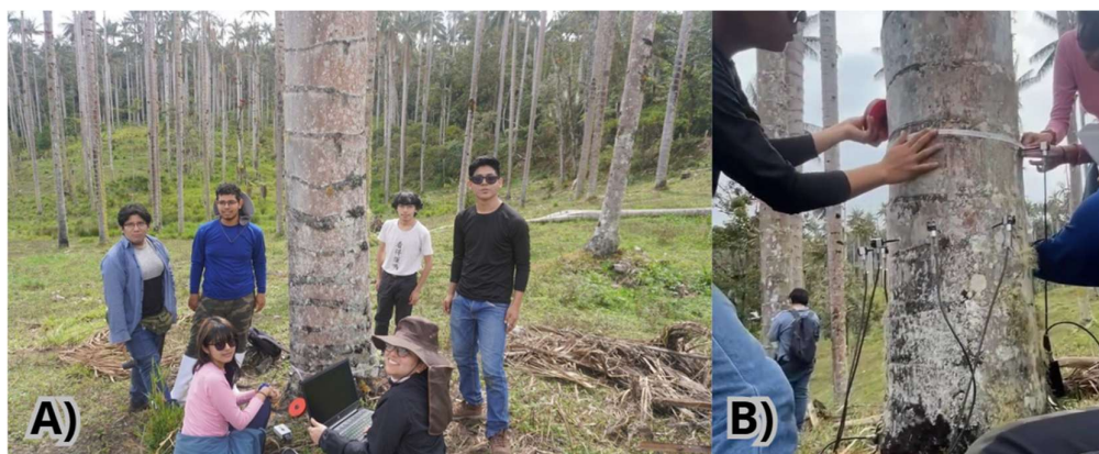
Figure 3. A) Field activities and configuration of the ArborSonic 3D (AS3D) sonic tomograph on palm individuals. The research team is shown conducting field measurements, and B) the installation of the instrument on the stipe, illustrating sensor placement and the measurement procedure for correct setup.
