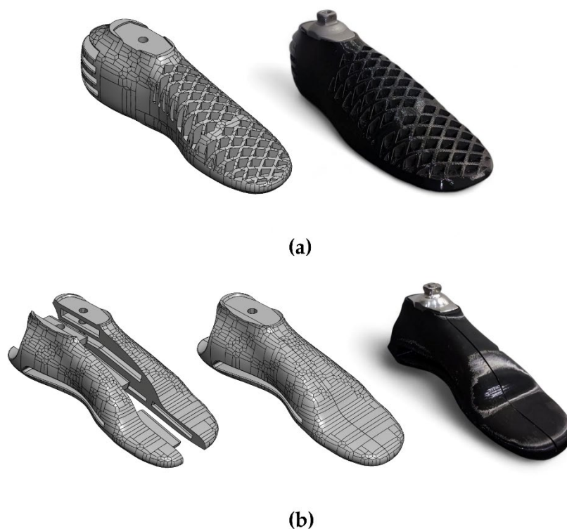
Figure 1. 3D models and photographs of the developed and fabricated 3D-printed prosthetic feet: (a) Model 1; (b) Model 2.
