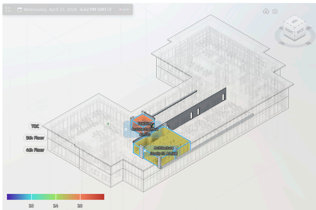
Figure 6. Monitored Spaces' live heat map illustrating live temperature variation based on the defined ASHRAE guided acceptable comfort range.
