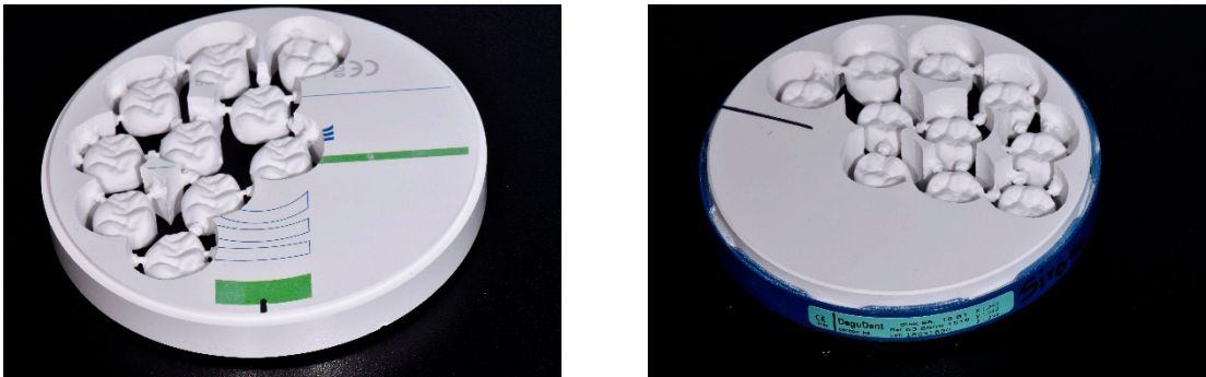
Figure 2. Restorations on CAD-CAM disks of zirconia dioxide before sintering.
