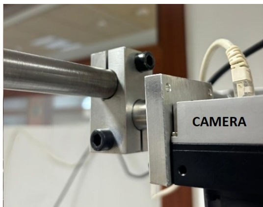
(a) Mechanism for precise adjustment of camera pan and tilt
