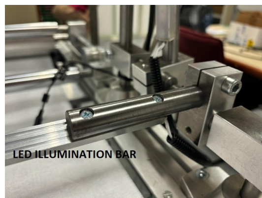
(b) Support system for LED illumination height and angle control
