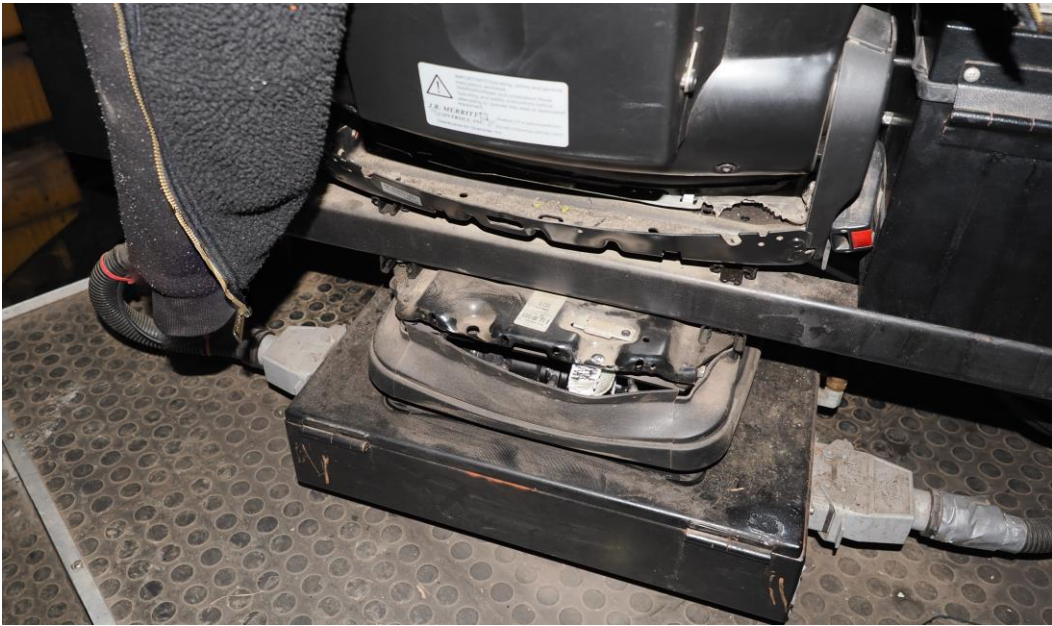
Figure 3. Operator seat spring system (rear view, bellows partially removed) with metal attachment bar of the side consoles mounted between seat pad/back rest and spring system and fixated on rotating platform. (© E. Johanning).
