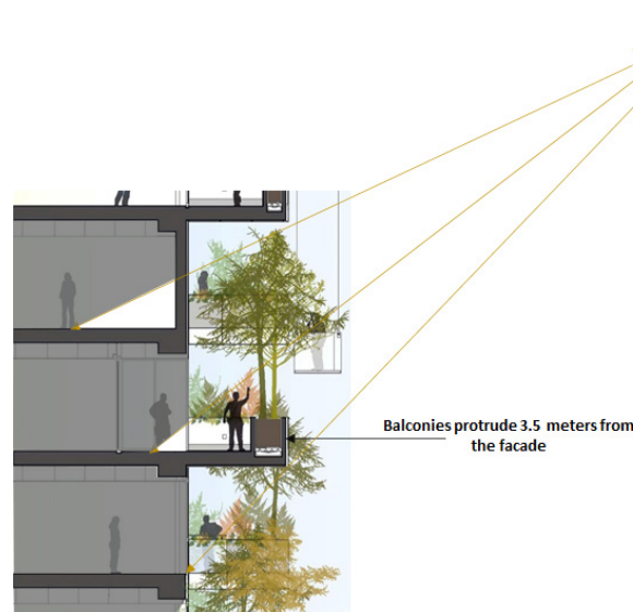
Figure 8. Large, cantilevered balconies, lush greenery, and tall trees block sunrays and natural daylight from Bosco Verticale's indoor spaces. (Sketch by author).
