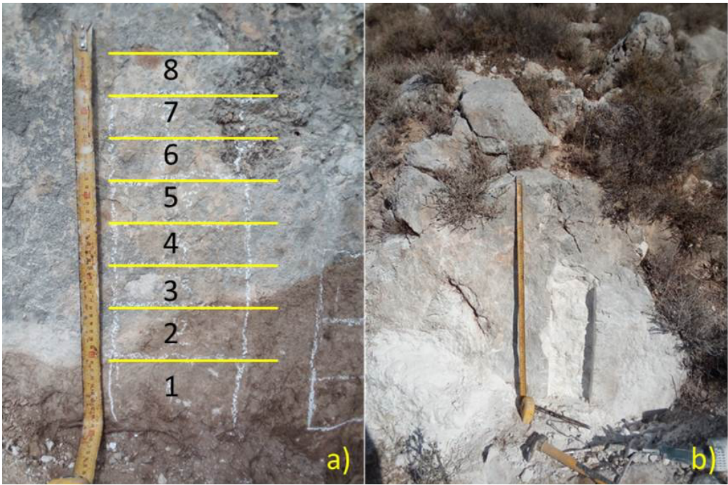
Figure 9. a) The fracture planar surface in the vicinity of the Kourouklata landform and the samples, extracted by tile-cutting wheel in 5 cm intervals. The surface is about 1 m high. b) The planar surface after the samples were cut out.
