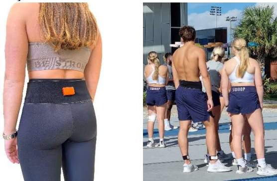
Figure 3. Utilised inertial measurement unit (IMU). a) The Xsens MTw Awinda IMU (orange) is placed in the athlete’s lumbar region near the S1 vertebra using a comfortable, wide Velcro strap (black) put around the athlete’s waist. b) The rest of Velcro strap is then put on top of the IMU to further fix its position, as can be seen for the shirtless male athlete in the front.
