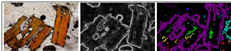
Figure 3. Original, low resolution thin section image of a biotite sample (left), edge detection (center), segmented regions (right).
