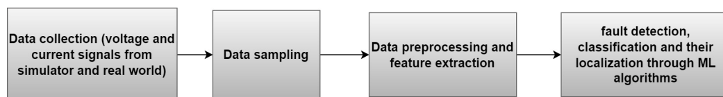
Figure 2. An Overview of TL Fault Detection and Localization in power transmission networks.
