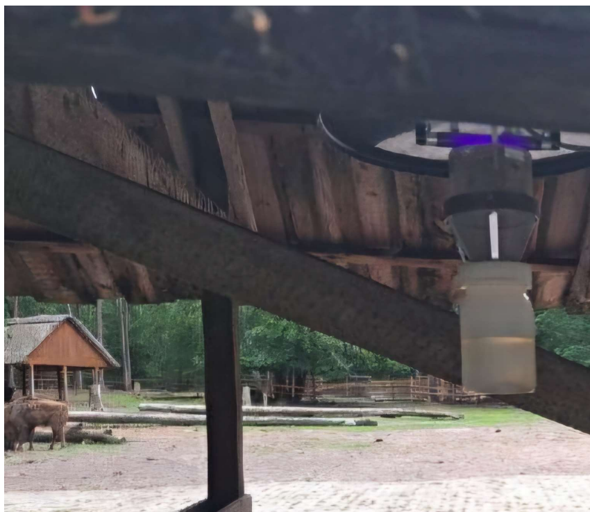
Figure 2. UV-light trap CDC 1212 (John W. Hock Company, Gainesville, Florida, USA) for Culicoides spp. collection installed at the European bison enclosure of Wolin National Park (WNP, Poland in 2024.
