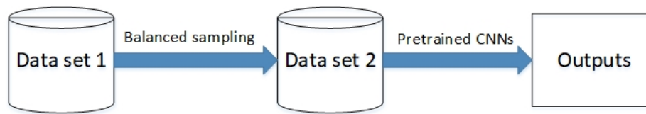
Figure 2. The proposed image classification framework for images acquired from visual traffic surveillance senso.
