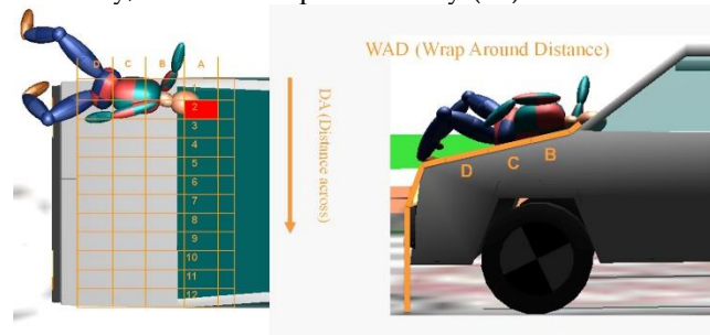
Figure 5. Estimation of the head-on-vehicle front-end impact cell from the reconstruction using PCCrash®
