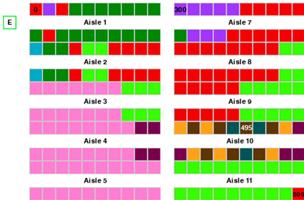
Figure 13. Effect of Picker Location (set to storage node with id 495) on mapping of k-Means Clusters to the Physical Warehouse Layout.
