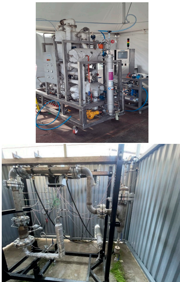
Figure 5. Pilot units for producing hydrogen-containing gas by combined matrix reforming. Gas capacity of up to 5 m 3 /h and an operating pressure of up to 2.5 MPa.
