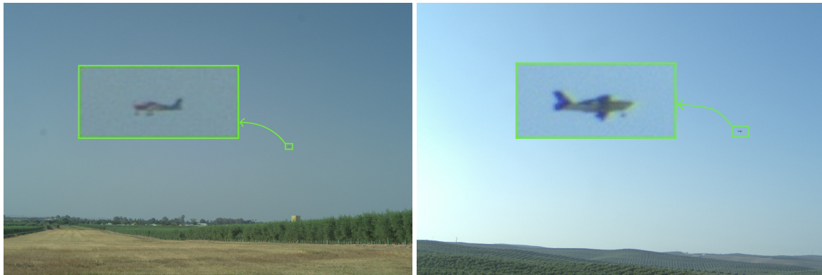
Figure 1. Images from our dataset, captured from the ground-based system, showing a small aircraft (SOCATA TB9) flying at a distance of two kilometers. Image resolution: 5472x3648 (20 MP); angle of view: 32.9° (horizontal) and 24.8° (vertical). Long-range detection poses a challenge to both image and audio-based strategies.
