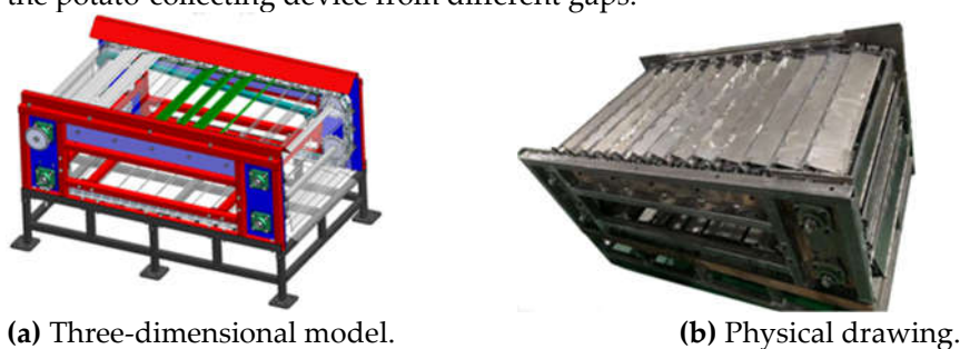
Figure 1. Movable rotating plate type grading device for potato.
