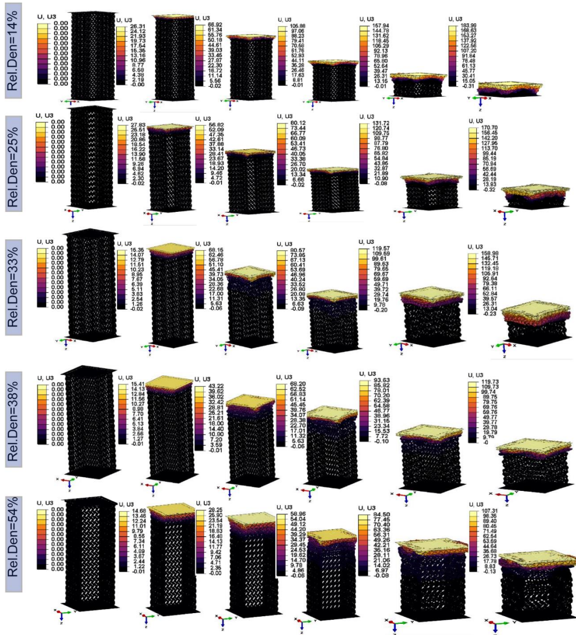
Figure 17. Maximum displacement contour result from simulation of Lattice Crash Box at Impact Speed of 15600 mm/s for 12.5 ms with Relative Densities of ; a) 14%, b) 25%, c) 33%, d)38%, and e) 54%. .
