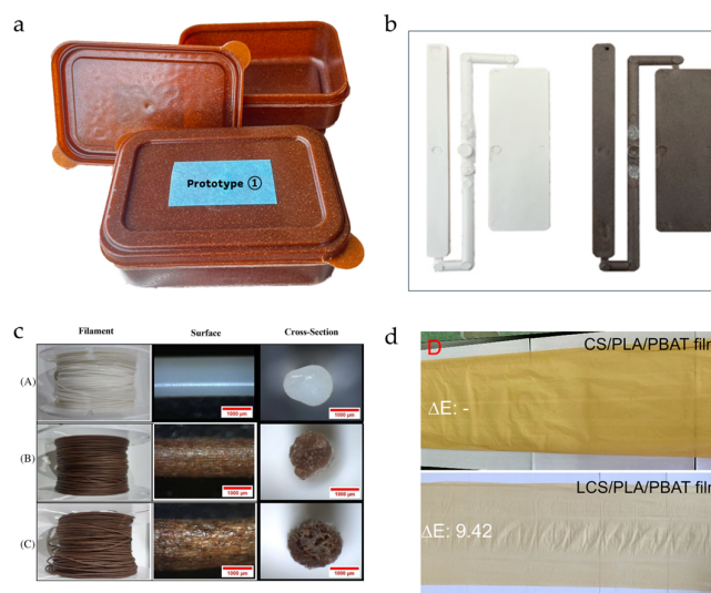
Figure 11. Prototype of biodegradable food containers (a) and biocomposites samples (b) obtained for injection molding; biocomposite filament for 3D printing applications (c); biocomposite film for food packaging applications (d). Reprinted (adapted) with permission from [67,77,87,91].
