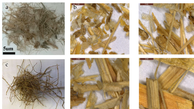
Figure 5. Close-up photos of abutilon indicum (a), corn stalk (b) and date palm (c) fibers. Reprinted (adapted) with permission from [96,100,118].
