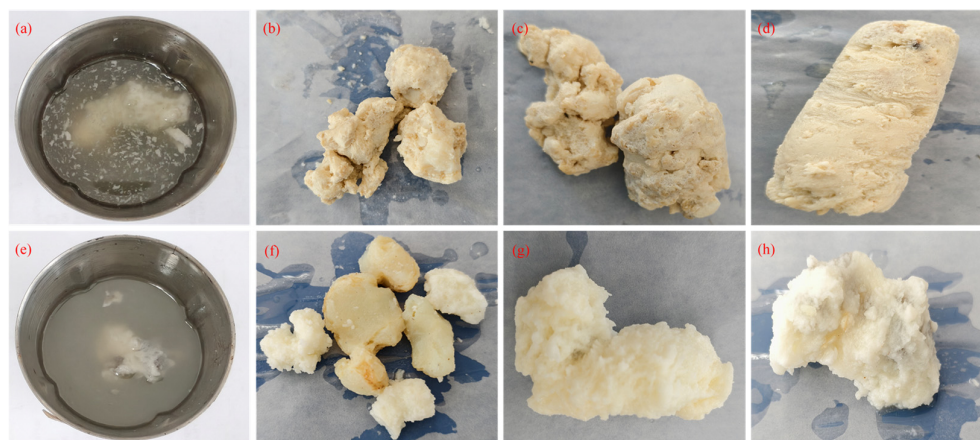
Figure 10. Compatibility of the RMFL(BPEI 10000 )/CFWBDFs with Ca 2+ and Mg 2+ . (a)-(d) Compatibility of BPEI 10000 with different concentrations of calcium chloride; (e)-(h) Compatibility of branched polyethyleneimine with different concentrations of calcium bromide.
