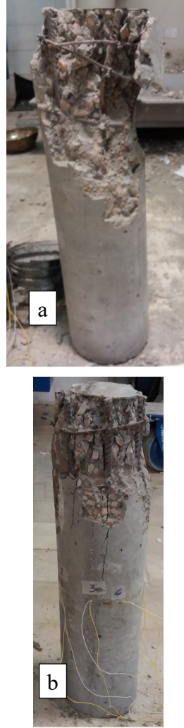
Figure 6. Failure of two columns under axial loading: (a) CP-P75 column; (b) SP-P75 column.
