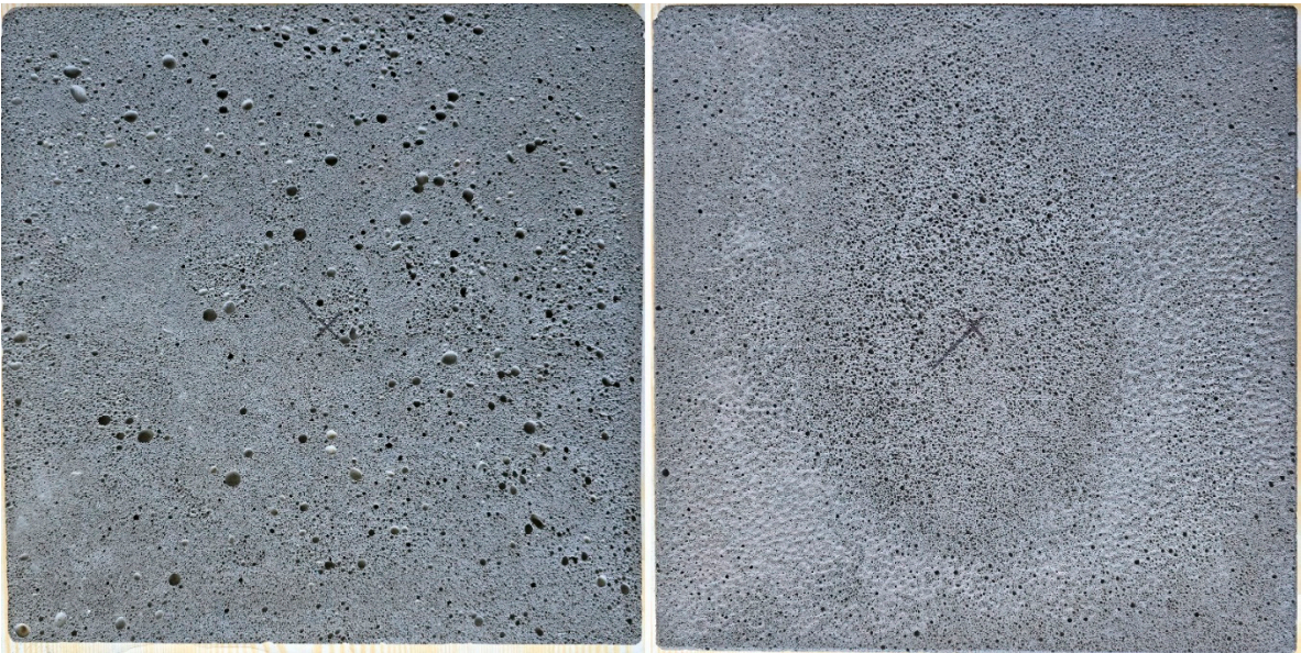
Figure 5. Real size polished specimen (300 x 300 x 30 mm) based on series FG15-AA. Top surface (Left) and bottom surface (right).
