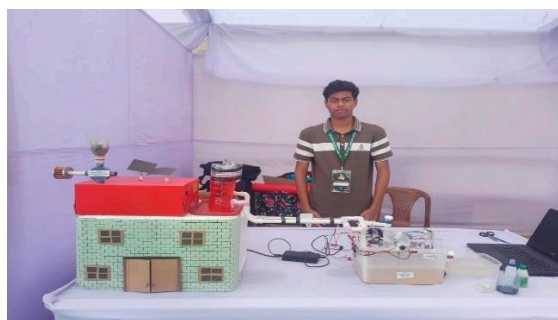
Figure 1. The complete operational prototype of the “Integrated Eco-Factory,” demonstrating the synchronization of the model factory unit (left), the waste-heat recovery system (center), and the hybrid water treatment unit (right).
