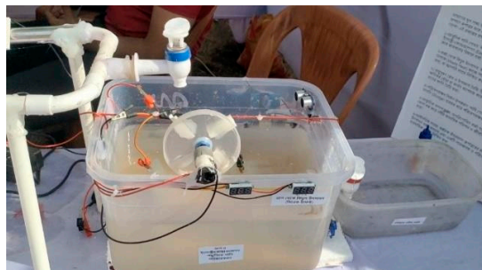
Figure 6. Close-up view of the operational unit: The hybrid chamber combining the Micro-Hydro turbine and Electrocoagulation electrodes.
