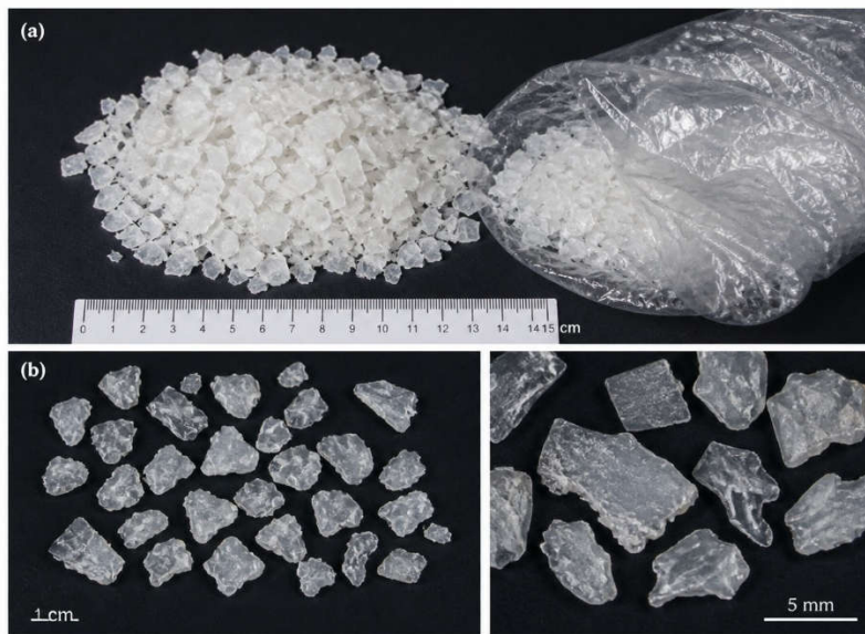
Figure 2. Crushed recycled low-density polyethylene (LDPE) used as partial fine aggregate replacement in mortar. (a) General view of the material with particle size < 0.90 cm. (b) Particle detail showing irregular geometry, smooth surfaces, and characteristic size distribution.
