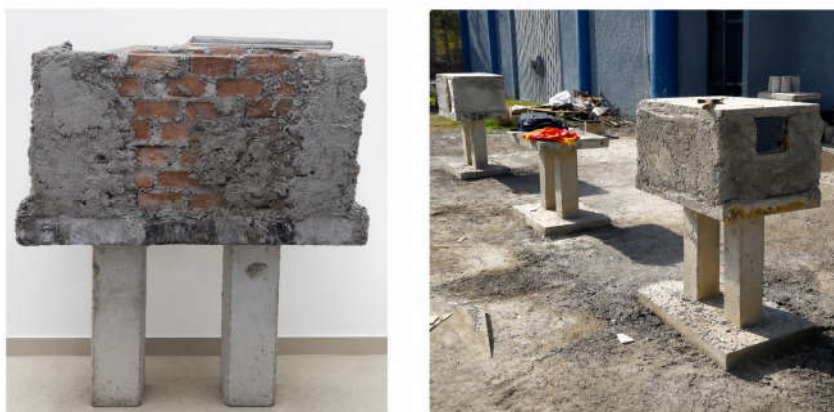
Figure 6. Construction and coating of the scaled chambers.
