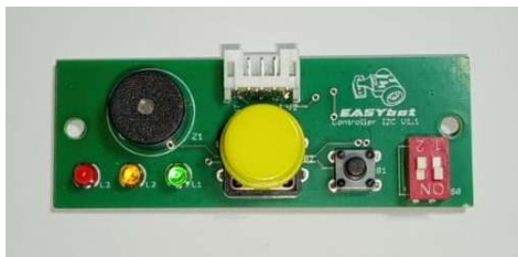
Figure 14. Photograph of the EASYbot IO Controller module (MCP23008-based I/O expander).
