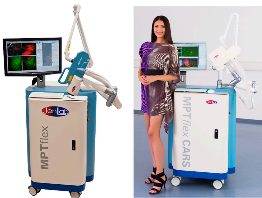
Figure 5. Multiphoton tomographs MPTflex and MPTflex -CARS based on a water-chilled tunable femtosecond Ti:sapphire laser, beam delivery through an optical arm, and the 360° imaging head with up to four photon detectors for the measurements of two-photon excited autofluorescence, SHG, and RAMAN/CARS signals of lipids and water.
