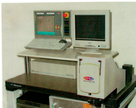
Figure 4. The first two-photon skin imaging device: multiphoton tomograph. This prototype was delivered to the Beiersdorf AG in Hamburg in 2001.
