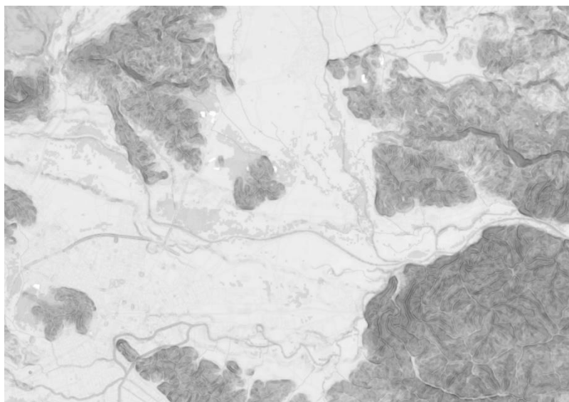
Figure 8. Spatial error model of the DEM, Ljubljana, Slovenia (area of 20 x 15 km): Darker shades indicate errors up to 8 m.
