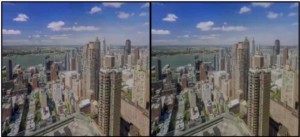
Figure 6. Preview of compression effects for frame 200 with QP=43 of the test video [61] (viewed from the left: the image compressed by pure AVC, and the image processed by ADNN and compressed by AVC).
