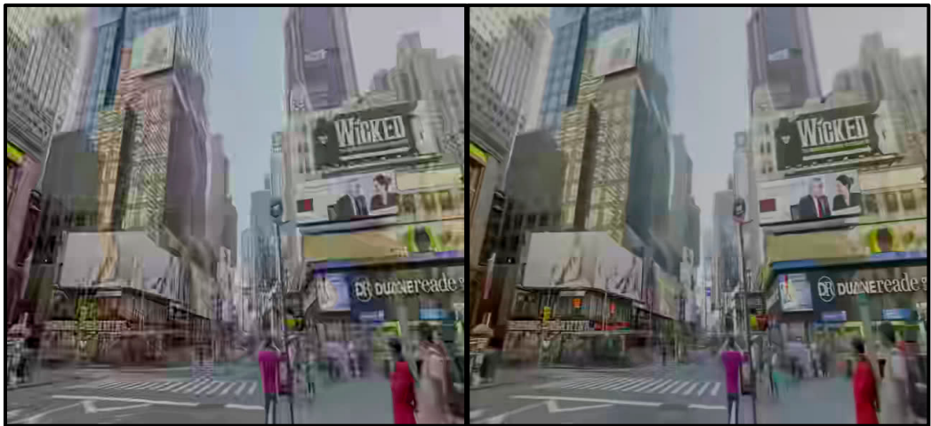
Figure 14. Preview of compression effects for frame 600 with QP=47 of the test video [61] (viewed from the left: the image compressed by pure HEVC, and the image processed by ADNN and compressed by HEVC).
