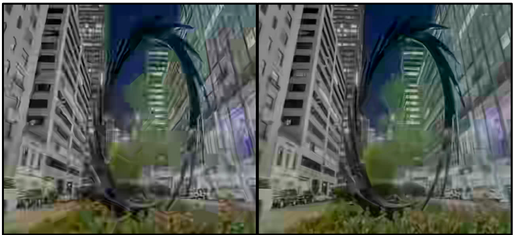
Figure 15. Preview of compression effects for frame 800 with QP=51 of the test video [61] (viewed from the left: the image compressed by pure HEVC, and the image processed by ADNN and compressed by HEVC).
