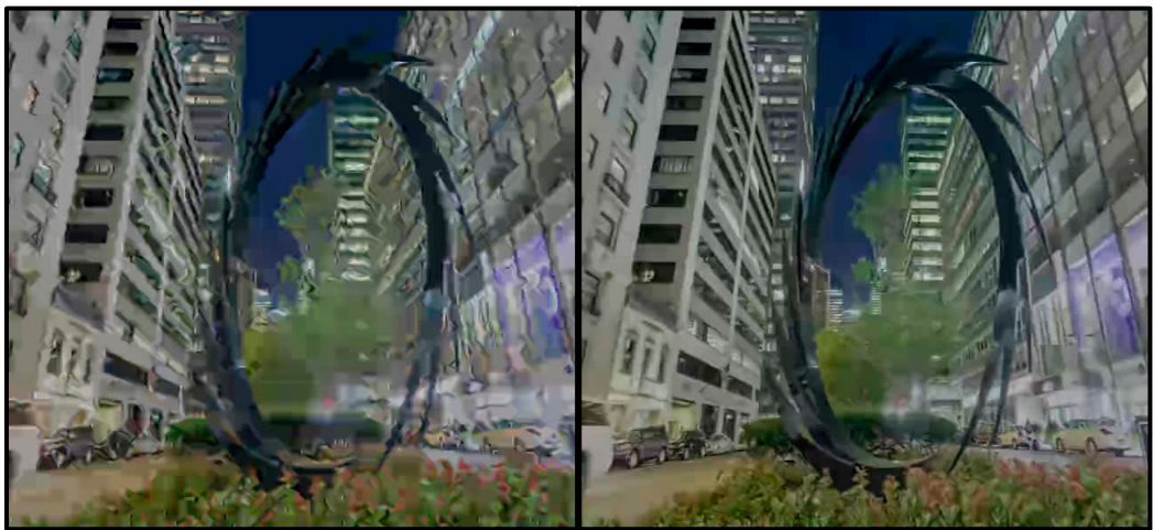
Figure 8. Preview of compression effects for frame 800 with QP=51 of the test video [61] (viewed from the left: the image compressed by pure AVC, and the image processed by ADNN and compressed by AVC).
