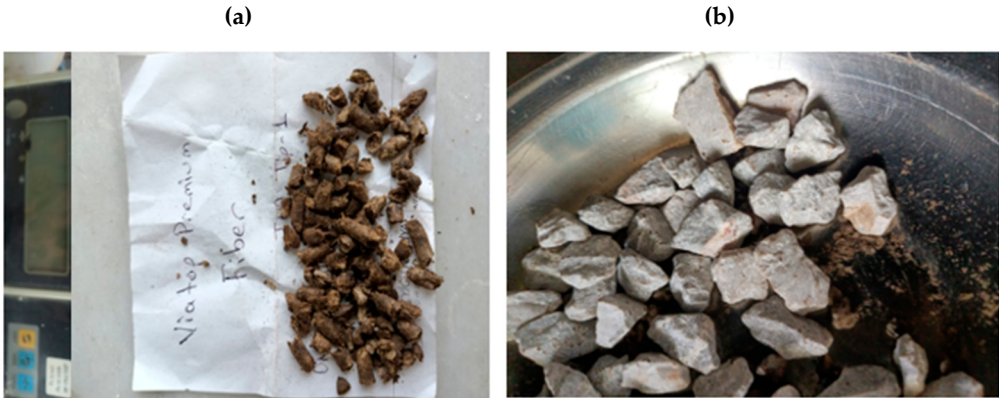
Figure 2. (a) Viatop premium fiber, (b)Fiber fragmentation.
