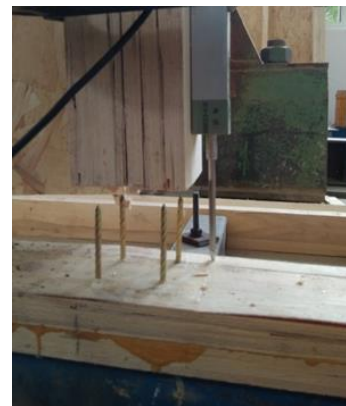
Uplift of Stud on One Side of Door Opening
