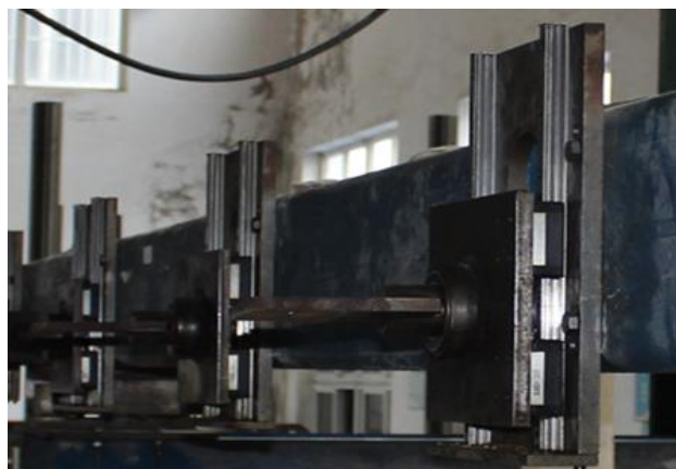
Figure 5. Out-of-plane Loading Beam.
