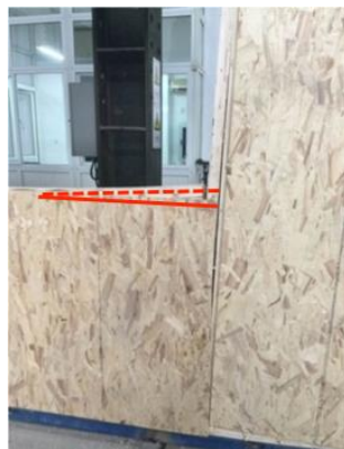
Torsion of Sheathing below Window
