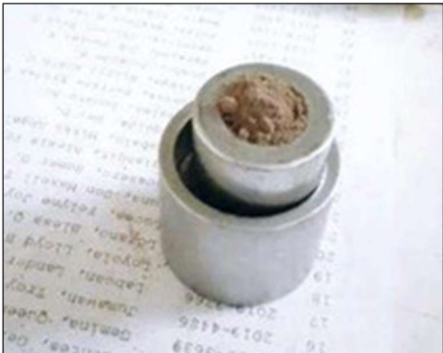
Figure B.2.2.1. Placing 4 grams of pulverized aged sample into the pelletizer.
