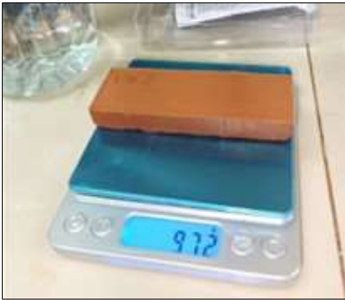
Figure C.1.1.1. Post test bar drying and firing weighing.
