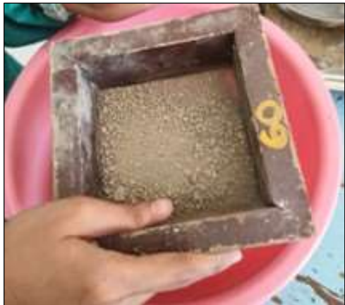
Figure B.1.2. Clay sample preparation: 60-mesh sieving.
