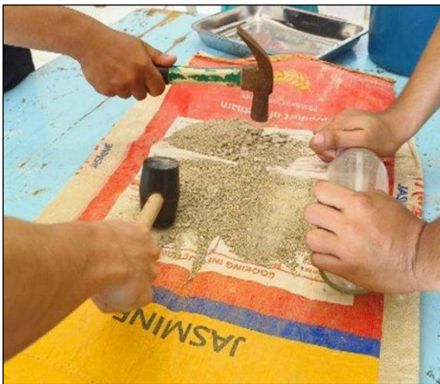
Figure B.1.1. Clay sample preparation: pulverizing.
