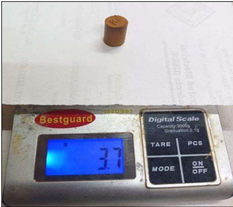
Figure C.1.1.2. Post pellet drying and firing weighing.
