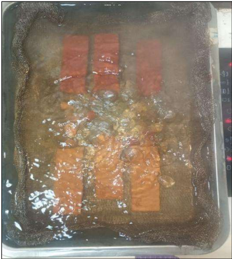
Figure C.1.2.1. Boiling of samples for water absorption test at 100°C.
