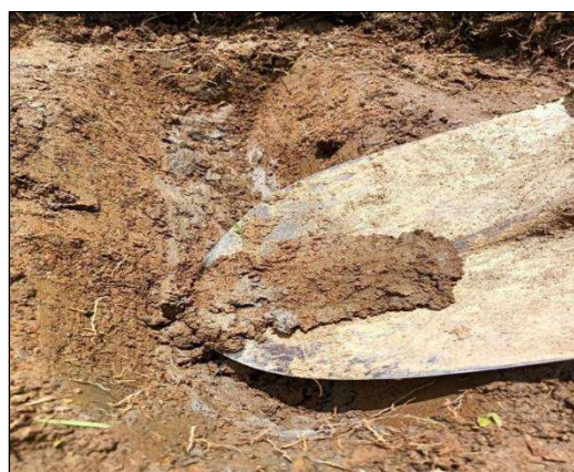
Figure A.1.3. Collecting four kilograms of sample at each sample point.
