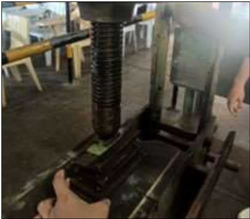
Figure B.2.1.2. Hydraulic pressing at 40N of controlled force.
