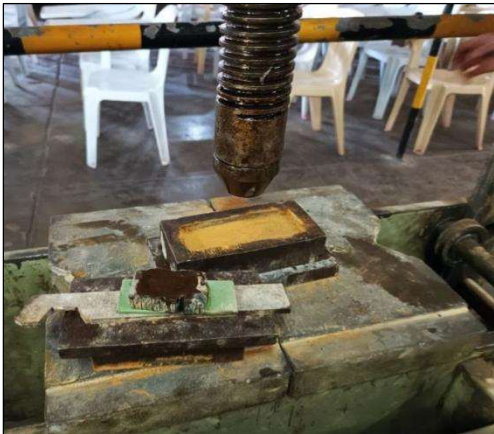
Figure B.2.1.1. Containing the mold 100 grams of pulverized clay samples.
