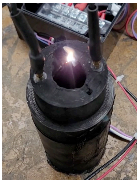
Figure 1. Inductive Pyrolysis of 3-D Printed ABS Fuel.
