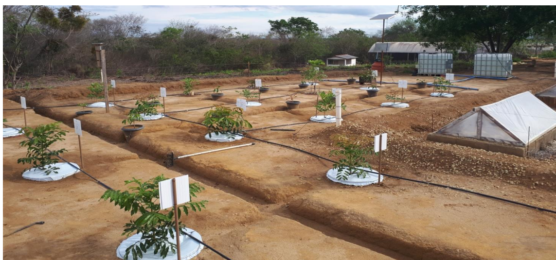
Figure 2. Field experiment with distribution of drainage lysimeters in the experiment area.
