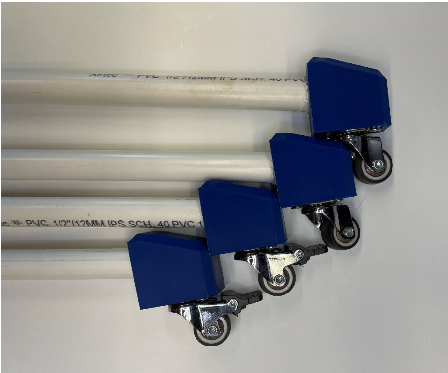
Figure 7. Caster wheels fitted to feet.
