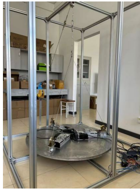
Figure 7. Cable-driven parallel mechanism prototype model.
