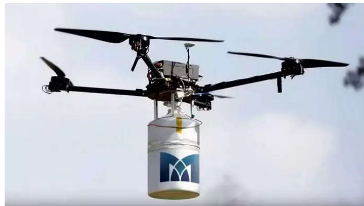
Figure 5. The liquid hydrogen storage fuel cell drone from Meta Vista.
